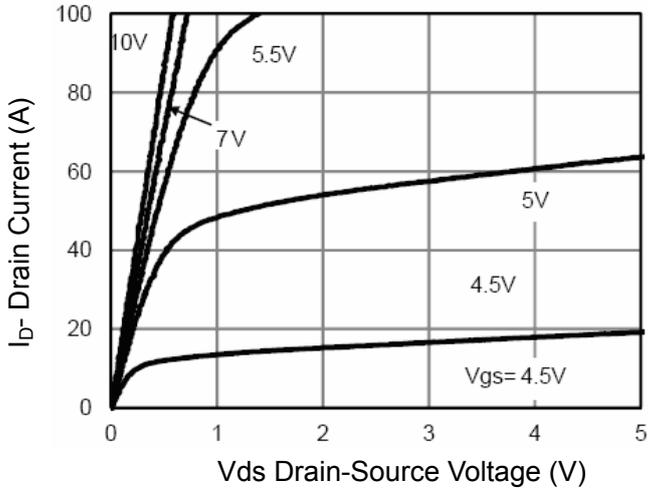
Figure 1 Output Characteristics
