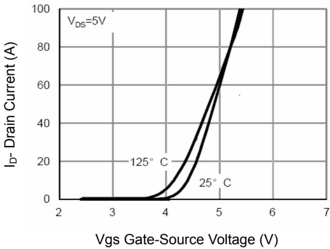
Figure 2 Transfer Characteristics
