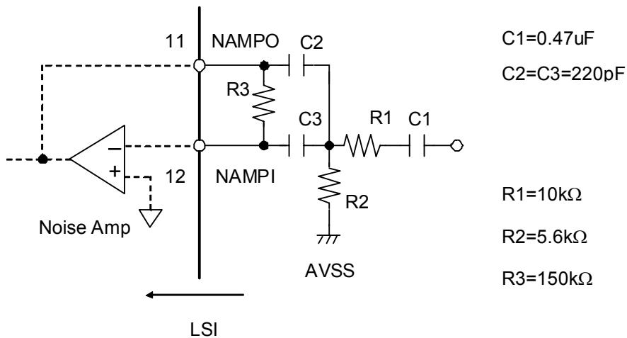
$$(1) \quad f_0 = \frac{1}{2\pi\sqrt{R_3(R_1//R_2)C^2}}$$
