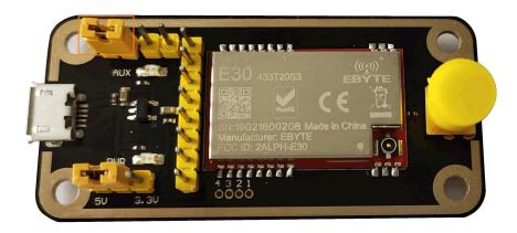
As shown above connect to jumpers (5V power supply mode 2), see function details from E30 UART module manual.
