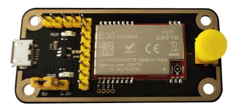
As shown above, connect to jumpers (5V power supply mode 3), see function details from E30 UART module manual.
