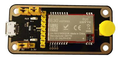
As shown above connect to jumpers(5V power supply, mode 0), both E30-433TBL-0 are configured this way, open serial port, for data TX and RX, and AUX indicator is blinking.
