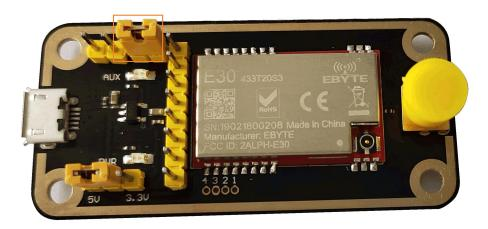
As shown above, connect to jumpers (5V power supply, mode 1) see function details from E30 UART module manual.
