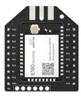
1. Used for testing and developing the Chengdu Ebyte E180-2G4Z20SX wireless module, E180-2G4Z20SX-TB has been pre welded with E180-2G4Z20SX, see details
