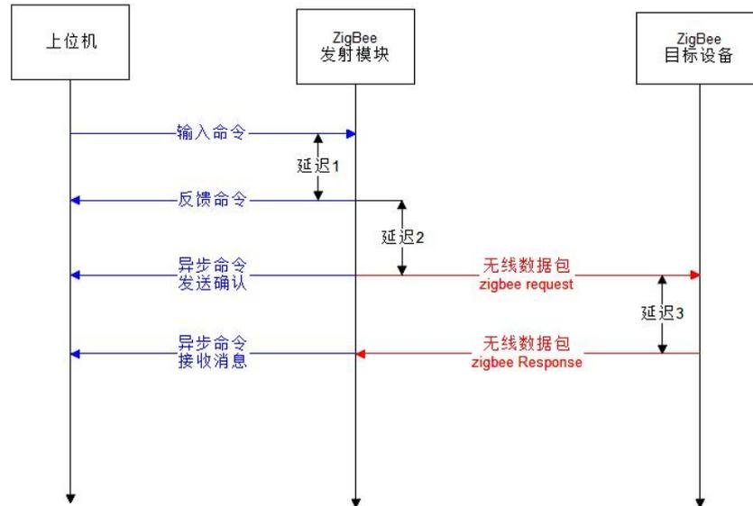
When the module sends network management commands and ZCL send commands by broadcast, due to the impact of broadcast flooding, the send confirmation will be triggered 1 second after the feedback command. Therefore, it is recommended that the sending interval be greater than 1 second when using this module for broadcast or multicast.
