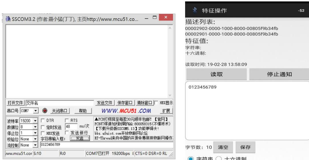
6. Click the fff2 channel, and click "Write", fill in and send "0123456789", you can see the received data in the serial debugging interface.
