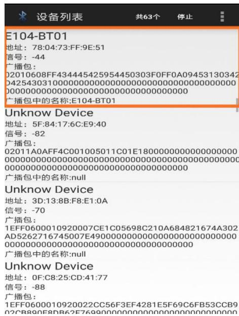
3. Click the device to connect, you can enter the service list interface of the Bluetooth device.
