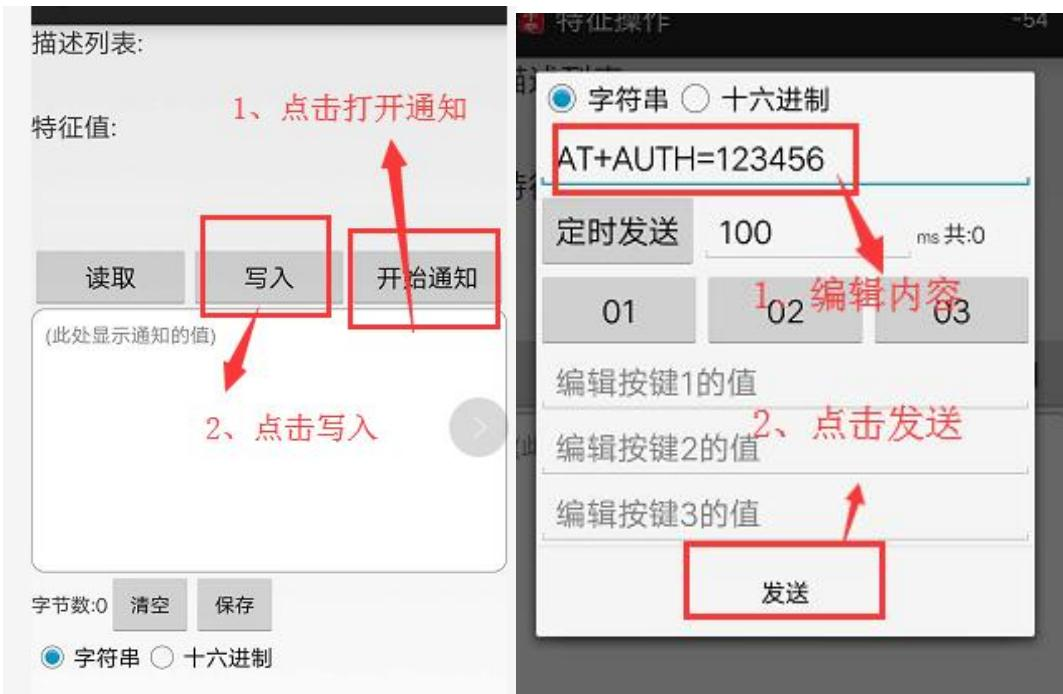
After the password authentication is successful, the return information "+OK" will be obtained. At this point, you can configure it in the air. Here is a demonstration of reading the device name.
