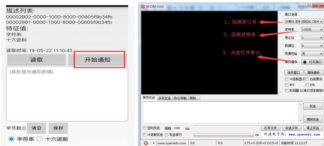
5. After the fourth step is completed, input data in the serial port, click Send can be received on APP.
