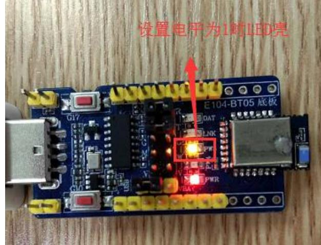
3、 Set PWM output, use AT instruction "AT + PWMFRQ = xx" to set the PWM cycle, and use AT instruction "AT + PWM1 = xx" to set the PWM duty cycle. The calculation method of PWM cycle is as follows: within the module, we set the precision to T=0.01ms, that is, the minimum cycle is 0.01ms. We can pass in parameters when setting, if need to set the cycle to 10ms, then t=T\*para, bring in T=0.01ms, t=10ms, and calculate para=1000
