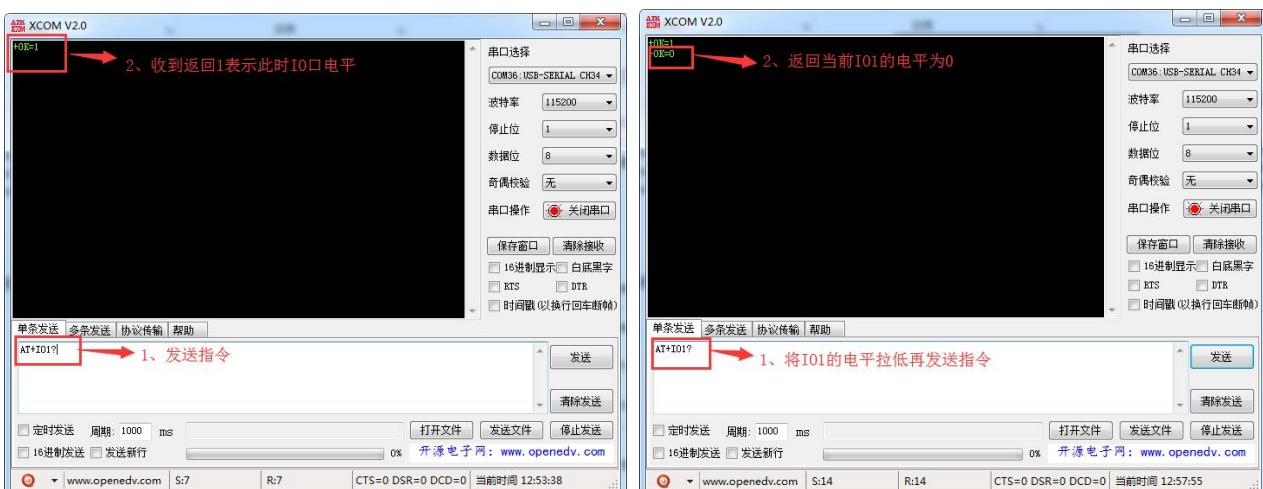
2、Set the IO2 output. Set the output level by using AT instruction "AT+IO2=xx". (This pin can be set as control pin according to the requirement, and the target device can be controlled by other devices or mobile APP)
