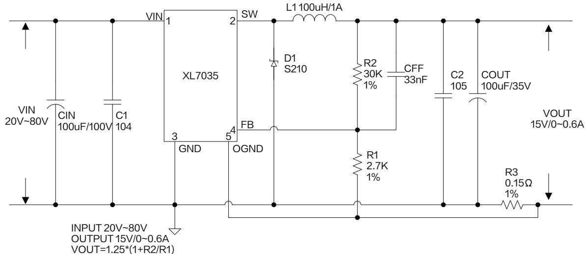
Figure7. XL7035 System Application (VIN=20V~80V, VOUT=15V/0.6A)
