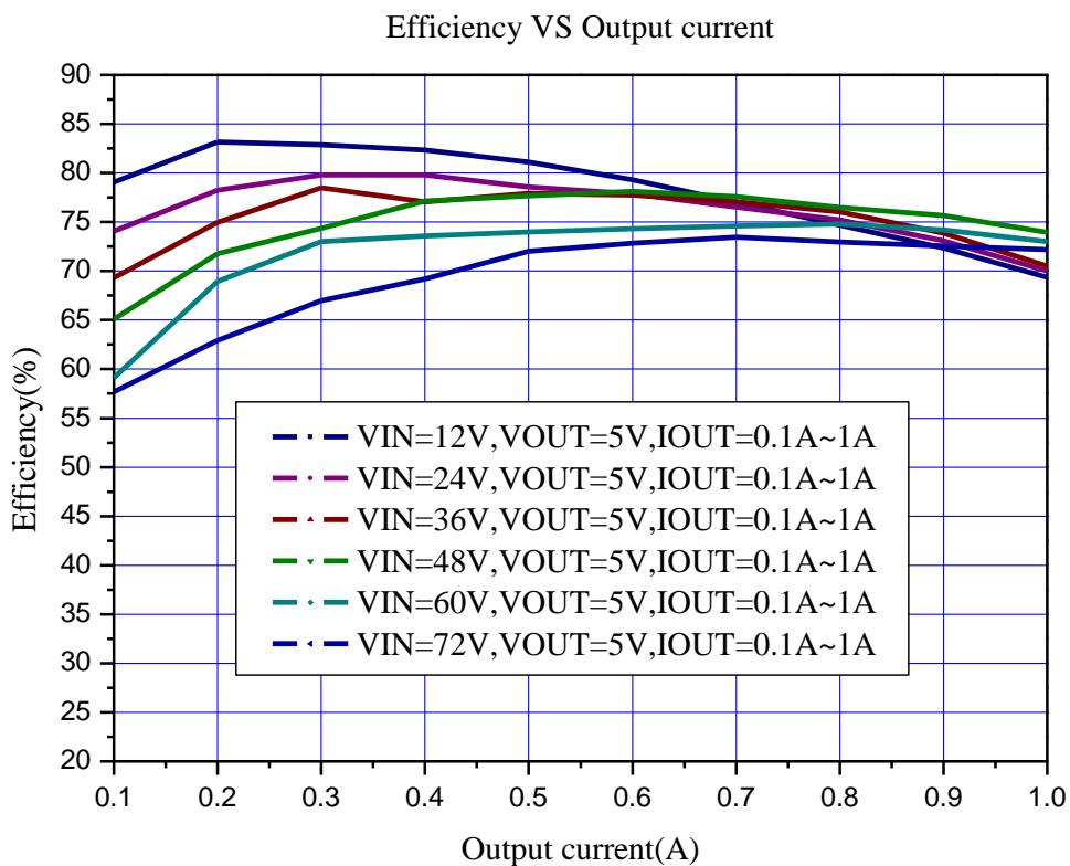
Figure10. XL7035 System Application (Efficiency VS Output Current)
