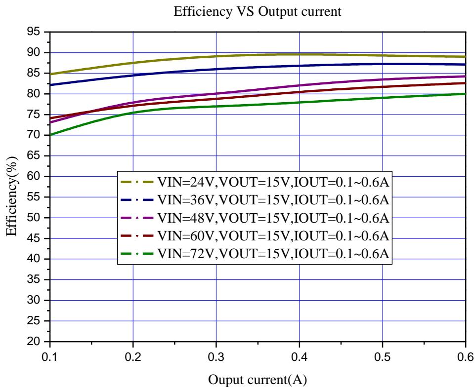
Figure8. XL7035 System Application (Efficiency VS Output Current)
