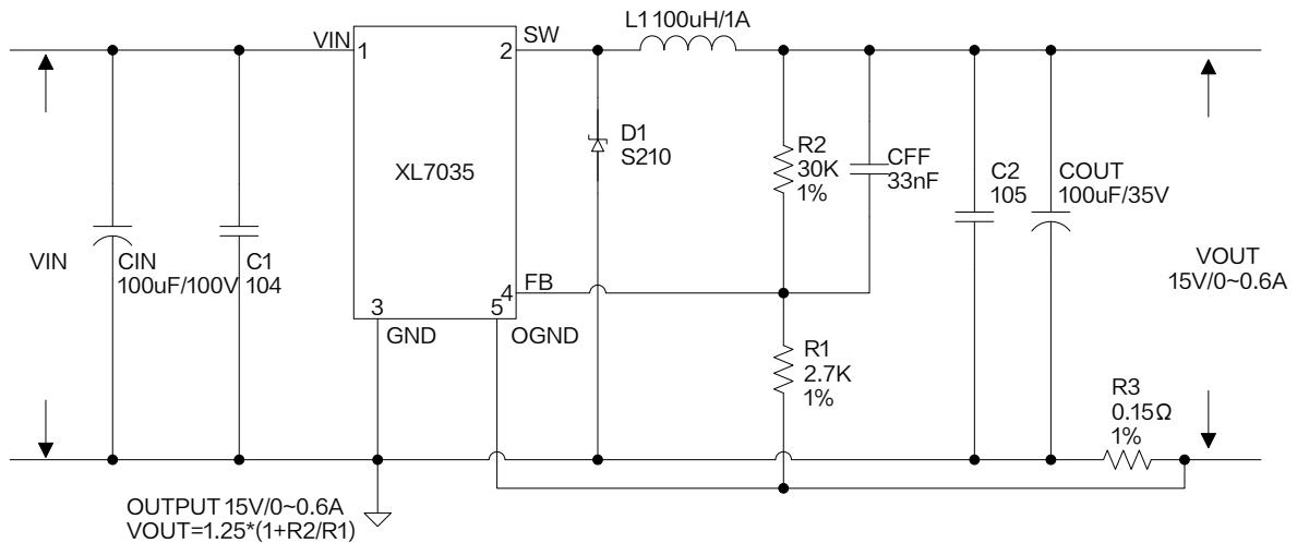
R3 for limit maximum output current, R3 choose 91 mohm in  $V_{OUT} \leq 5V$  application; R3 choose 150 mohm in  $V_{OUT} > 5V$  application.
