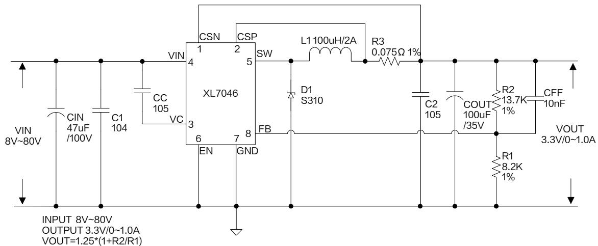
Figure11. XL7046 System Application (VIN=8V~80V, VOUT=3.3V, IOUT=0~1.0A)
