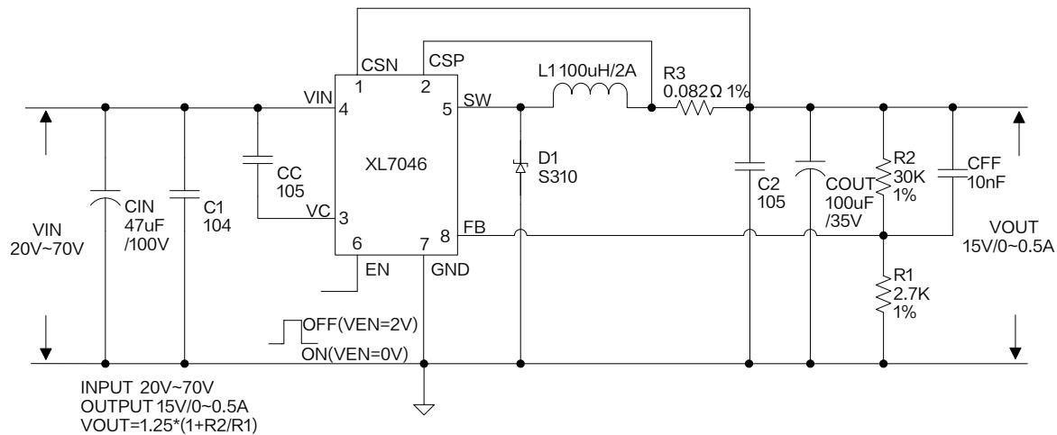
Figure8. XL7046 ON/OFF Mode Application (VIN=20V~70V, VOUT=15V, IOUT=0~0.5A)
