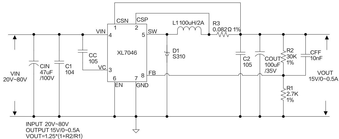
Figure7. XL7046 System Application (VIN=20V~80V, VOUT=15V, IOUT=0~0.5A)
