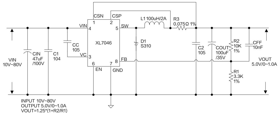
Figure9. XL7046 System Application (VIN=10V~80V, VOUT=5V, IOUT=0~1.0A)
