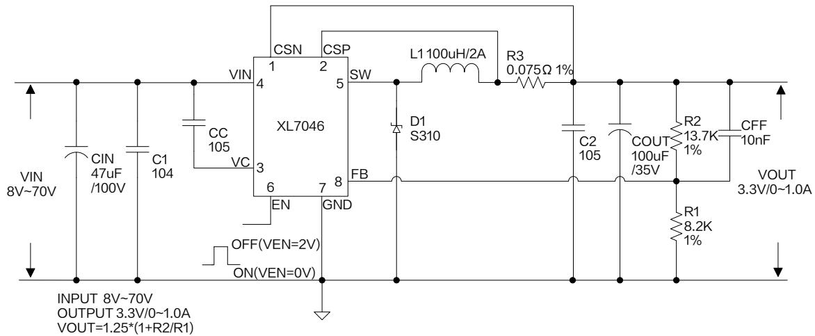
Figure12. XL7046 ON/OFF Mode Application (VIN=8V~70V, VOUT=3.3V, IOUT=0~1.0A)
