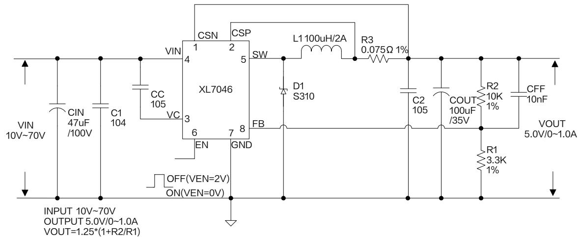
Figure10. XL7046 ON/OFF Mode Application (VIN=10V~70V, VOUT=5V, IOUT=0~1.0A)
